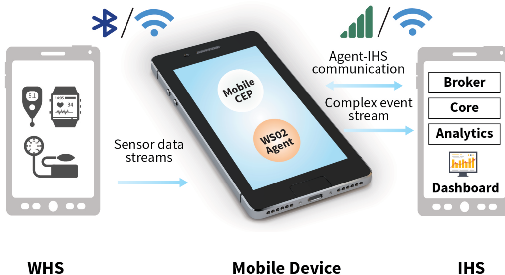
The figure (based on [1]) presents the architecture for a remote patient monitoring system. Wearable Health Sensors (WHS) send sensor readings to the mobile device, which uses the embedded Complex Event Processing (CEP) Engine to detect complex events and send them to the remote IoT Hospital Server (IHS) for further processing at the backend and notification.
