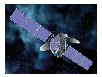
relative to Earth's surface by orbiting above its equator, with an orbital time matching Earth's rotation. From this position, TEMPO will be able to 'sweep' the entire continent once every hour – picking up incredibly small details. 'TEMPO's mission is to measure atmospheric pollution over North America hourly in the daytime, at a spatial resolution of around 10 square kilometers,' says Dr Chance.
