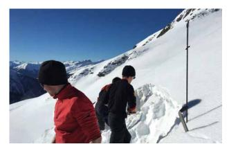
How does this work? Most back-country snow-goers carry an avalanche probe – a long, foldable pole which allows you find buried people in the loosely-packed snow following an avalanche. The volunteers take three measurements within a one-metre circle, calculate the average, and then enter this information into the Mountain Hub app. The app automatically includes their location and these data are sent in to a central server as soon as a wireless connection is established.
