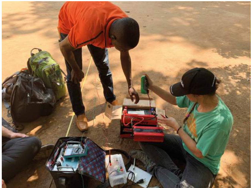
Mines Geoscientists Without Borders members deploy low-cost geophysical instrumentation for locating water at-depth with citizens in Benin, Africa.
