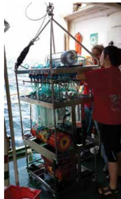
M. Pachiadaki and V. Edgcomb preparing submersible sampler developed at Woods Hole Oceanographic Institution that preserves gene expression samples in situ.
