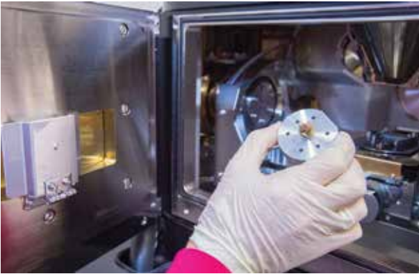
Gold sputtered separator material used in fundamental studies of battery
