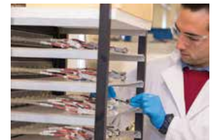
A battery scientist begins long-term performance testing on a sodium coin cell
