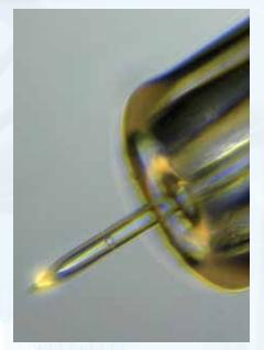
vacuum or pressure control for the space between the two tips, the space between the inner tip and the injection probe, and the space inside the injection probe, itself. Embryos are held firmly yet without damaging stresses by a ring of vacuum between the two tips. A brief pulse of vacuum inside the inner tip can aid in penetration as the injection probe is advanced. The Dracula system draws the injection surface taught, like the surface of a drum.
