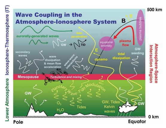
Energy and momentum are transferred from one point to another within the atmosphere-ionosphere system through the generation and propagation of waves. In the ionosphere wind perturbations associated with the waves can redistribute ionospheric plasma, either through the electric fields generated via the dynamo mechanism, or directly by moving plasma along magnetic field lines. Adapted from Figure 8.10, Solar and Space Physics Decadal Survey, National Academy of Sciences, 2012.
