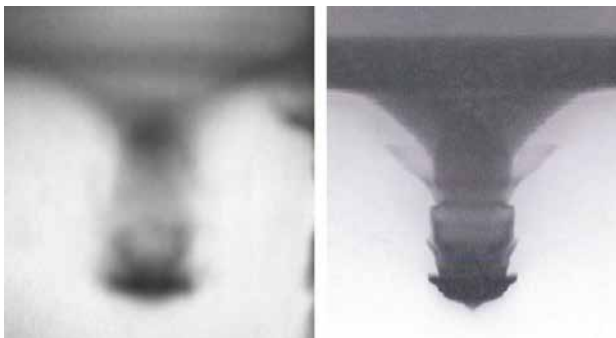
Simulated image (right) of the evolved target show similar evolution to the data (left). The dark band at the top of the image is the shock in the low-density foam and is moving up, away from the radiation source. The shock colliding behind the clump created a triangular band near the top of the image. At the bottom of the image is the dense clump and above the clump is a shock, moving away from the column of plasma.
