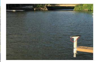
Dr Glazer's group develops and tests inexpensive dataloggers with integrated telemetry capabilities and adapts an appropriate level of sensor accuracy, precision, expense for the appropriate application. There's little need to deploy expensive conductivity sensors that can measure four decimal places of accuracy in a location that may experience a 30% daily fluctuation, if lower-cost sensors can provide more measurements in more places to better understand spatial questions.
