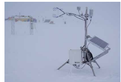
A sonic anemometer measuring near-surface turbulent energy fluxes at Siple Dome in West Antarctica. Credit: Dan Lubin.
