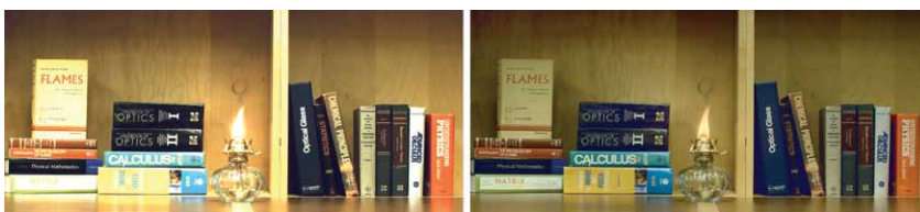
Single image from a video taken with a standard camera (left) and using I2R's near-real time high-speed HDR video technology (right)
