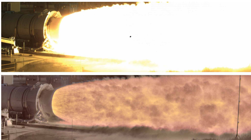
Single image from a high-speed rocket plume video taken with a standard video camera (top) and using I2R's high-speed HDR video technology (bottom)
