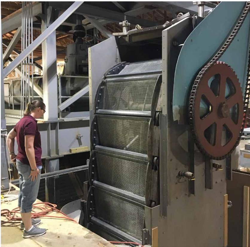
scale loss, continuous rotation of the screens, low-pressure spray washes, and fish return features with sufficient water flow and no large drops. Out of the available technologies, these fish-friendly travelling water screens are likely to be frequently used, because they can be easily retrofitted to existing water intake systems.
