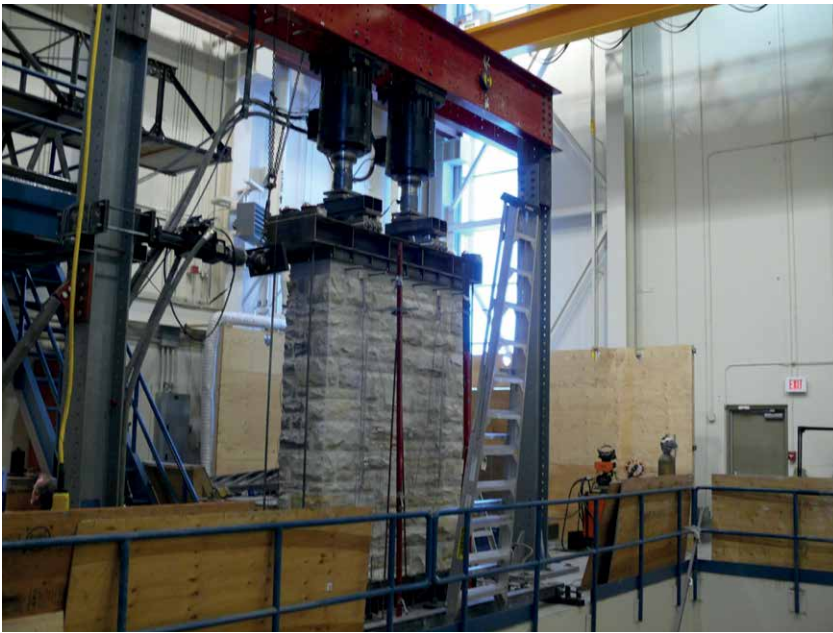
A wall in the in-plane test rig.
