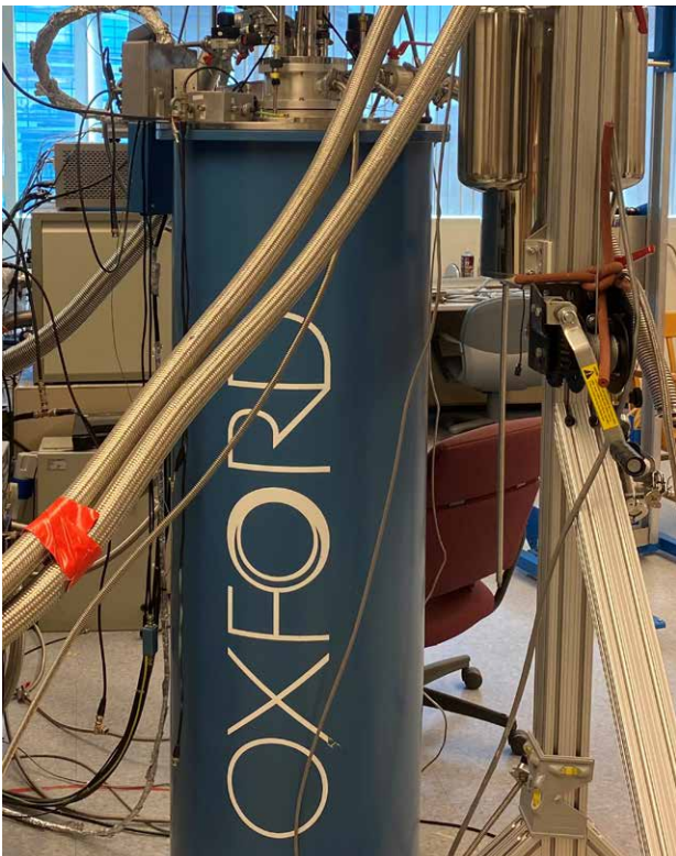
Oxford dilution refrigerator capable of producing temperatures down to 18 millikelvins. Credit Sergey Kravchenko
