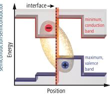
their atomic structures for the first time. Where the GaP/Si border previously seemed intermixed, images of the interface revealed a scale small enough to show abrupt boundaries between the solids. The team discovered that the defects introduced local regions of electric charge, ultimately determining the performance of the overall semiconductor.
