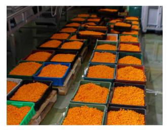
causing internal water to be driven to the surface where it evaporates. This process can also cause channels to open in the material as the water is removed, which in turn can lead to even faster drying times.
